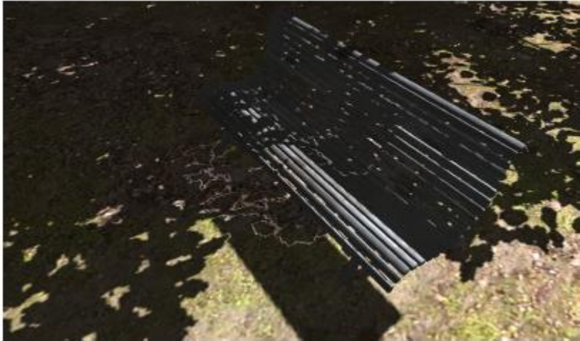
Figure 20: The penumbra areas from the tree leaves are incorrectly bleeding through to the shadow below the bench.
